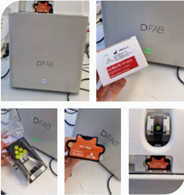
FIG. 4A-E The stereolithographic printer (DFAB®, DWS Systems, Italy) used in this case report. (A) The material used for manufacturing the crown and the abutment was an hybrid composite (Irix Max®, DWS Systems, Italy). This material is certified in Europe and US as definitive material; (B) the Irix Max® cartridge; (C) the material used here has three layers of colours thanks to the tilted stereolithography concept and the proprietary Photoshade® technology; (D) the cartridge and the printing plate in position; (E) the printer is ready for use.
