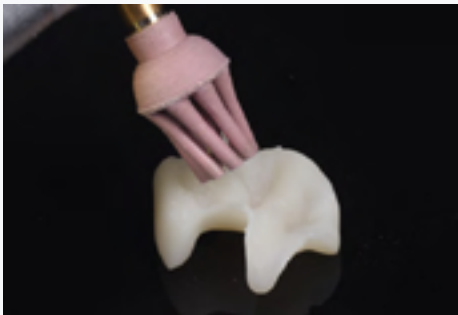
FIG. 12 A two-step diamond-impregnated polishing system is used to achieve the desired texture and lustre. First step: Use medium-grit tools to polish.
