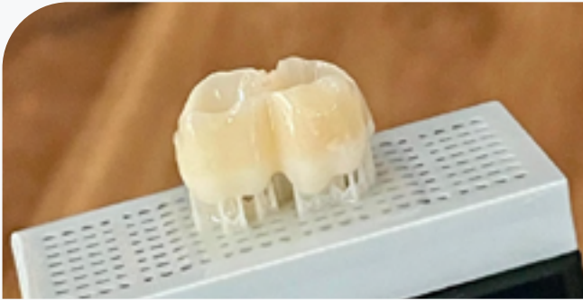
FIG. 6 Dfab restorations, as printed and still on the platform.
