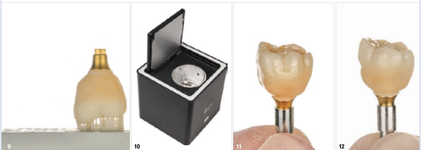
Fig. 9: Dfab-printed crown, still on the platform, after washing with 95% ethanol and drying. Fig. 10: Dcure post-polymerisation unit. Figs. 11 & 12: Finished crown cemented to the Ti-base with a dual-polymerising resin cement.
